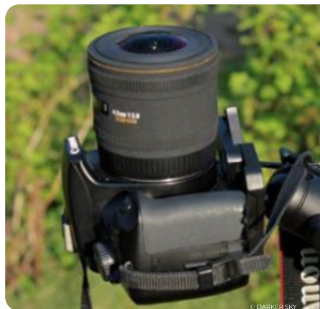
Figure 8: Sky Quality Camera (SQC, Canon 6D camera and Sigma fish-eye lens) installed in a protective housing.
