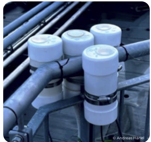
Figure 6: The housing of SQM-DLs and SQM-Ls.
